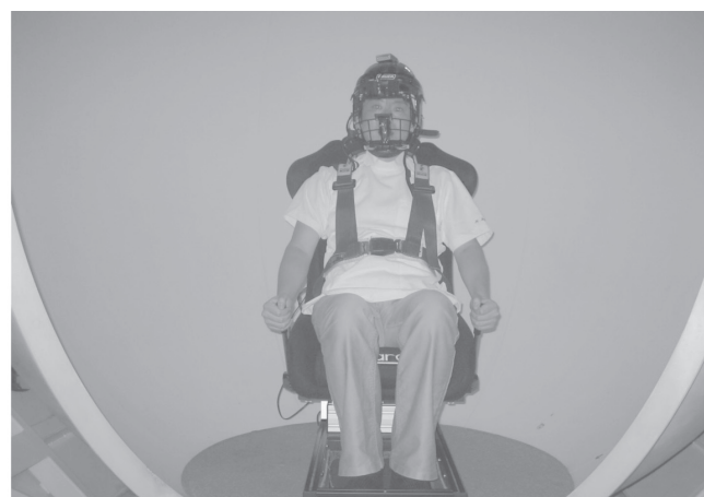
Fig. 1. Two infrared CCD cameras with cold filters for see-through vision were included in the whole head helmet with facemask. The cold filter was made of 31 layers of mutually laminated TiO 2 and SiO 2 . The subjects bit a bite bar integrated into the helmet to keep the position between the cameras and the subject's eyes constant.
