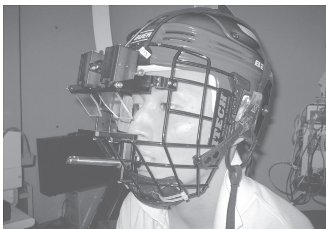
Fig. 1. Two infrared CCD cameras with cold filters for see-through vision were included in the whole head helmet with facemask. The cold filter was made of 31 layers of mutually laminated TiO 2 and SiO 2 . The subjects bit a bite bar integrated into the helmet to keep the position between the cameras and the subject's eyes constant.
